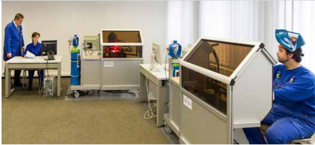
The GSI SLV Welding Trainer combines elements of hands-on education of welders and computer-based simulation to educate welders as realistically as possible
