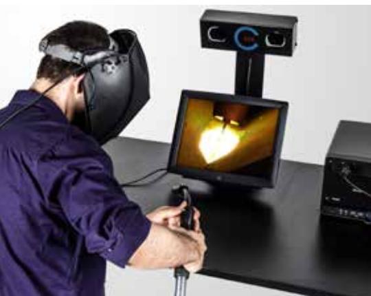
The Arc+ Welding Simulator is a training tool that powers lifelike virtual welding practice
