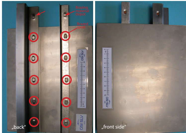
Demonstration sample for spot brazing steel, sheet thickness 1 mm
