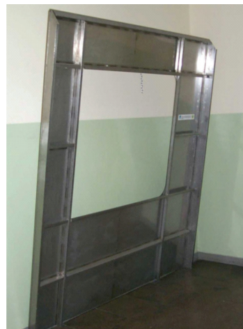
Lateral wall segment with stitch welds
