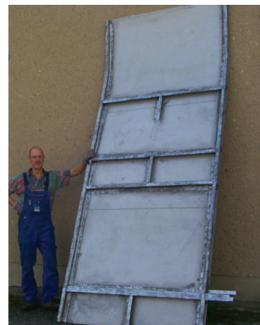
Segment with weaving and circumferential welds
